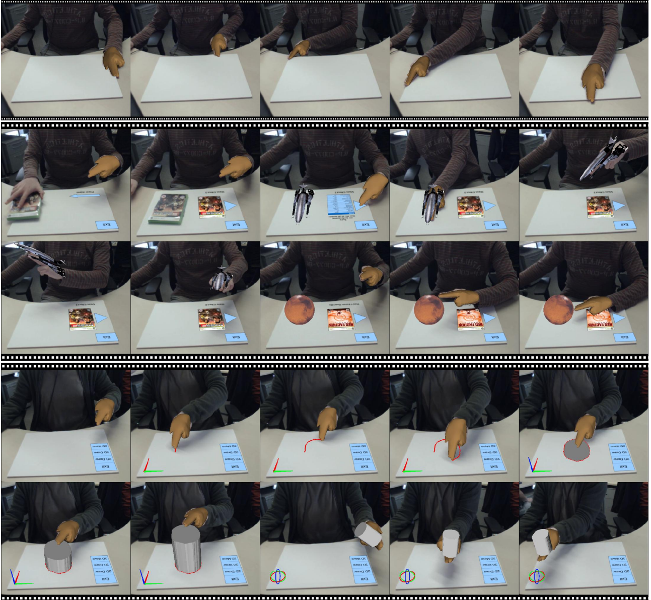
Figure 21: Example human-computer interface based on our tracker. Top filmstrip – calibration – the user marks a plane by moving the hand along the edges of the board. Middle filmstrip – the user places a DVD box on the surface, prompting the system to show facts about the DVD box and a 3D object related to it, which can be manipulated with the hand. For the first DVD, the user can interact with a 3D model of a starship. For the second DVD, the user can interact with a model of planet Mars. Bottom filmstrip – the user can draw on the 2D surface, transform the 2D drawing into a 3D object (by tapping inside it and lifting the hand) and pick up and move the 3D object.
