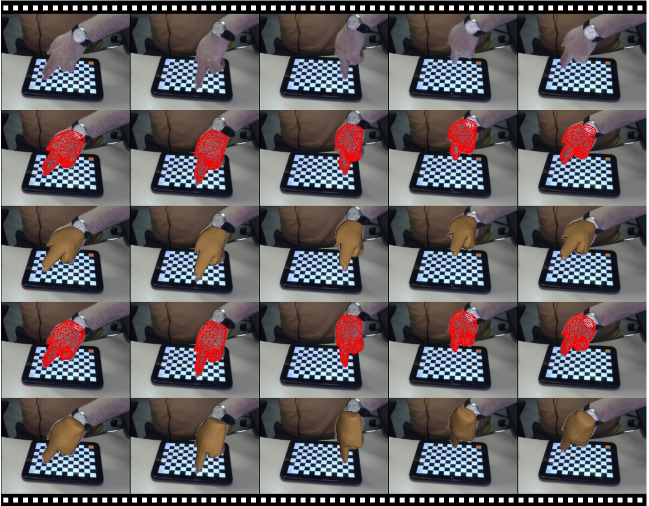
Figure 20: Example frames and results from the rotation accuracy test. Original image (first row), wireframe (second row) and full rendering (third row) results of our method, without the accelerometer, wireframe (forth row) and full rendering (fifth row) results of our method, with the accelerometer.
